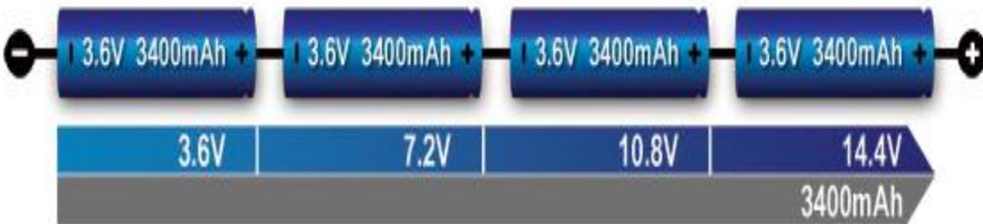
**Figure2: Series connection of four cells (4s).**
