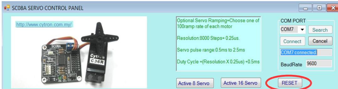
19. Extra information, User can directly click the link provided on SC08A Servo Control Panel for visit Cytron Technologies Website page. Other information also provided on Text Box which show on top of control panel.
