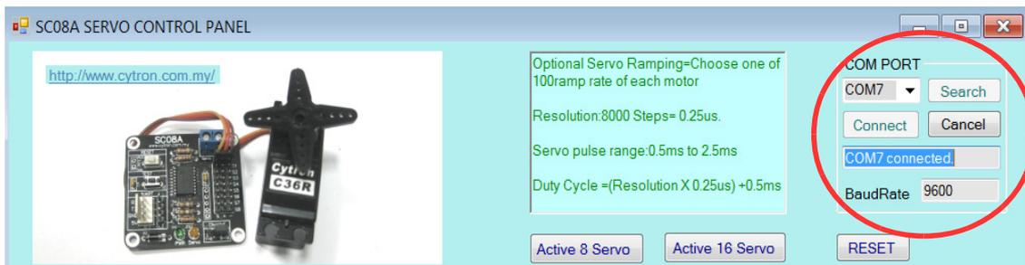
10. SC08A servo controller can be control 8 servo motors, but user also can expand another SC08A for control maximum 16 servo motor. So that, SC08A Servo Control Panel provide two icon which is “Active 8 Servo” and “Active 16 servo” for user select one of them.
