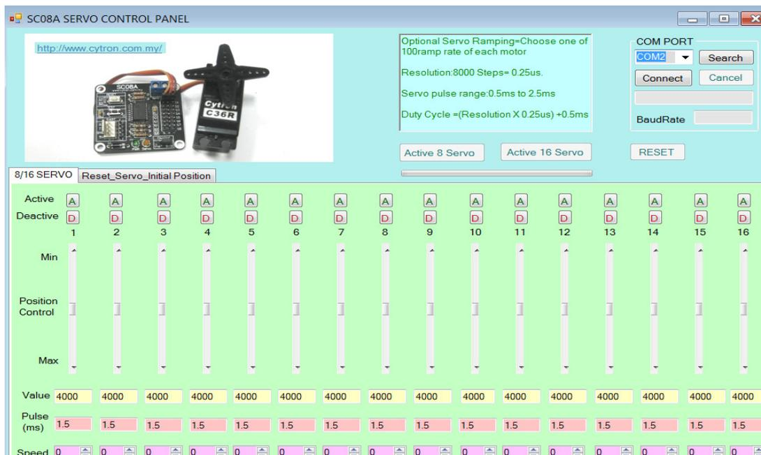
7. Ensure the UART port device connect to computer, click the “Search” icon for refresh the COM Port searching. Choose the COM Port by clicking the side bar, choose the last COM Port. Normally, the extra virtual COM port will be largest number port after drive installation. Click on it.
