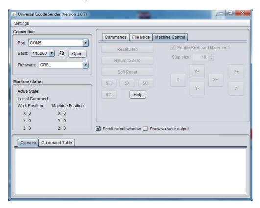
Click the "Machine Control" tab. Select the "Port" number which your Arduino board is attached to. Select 115200 as the Baud rate as this is the speed configured in "GRBL" firmware. Click "Open" button to start the communication for controlling this shield board.
