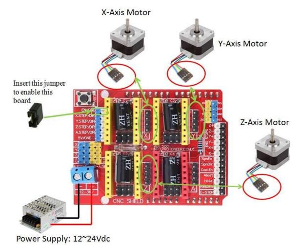
Your CNC Shield board is now ready to go for a test run, let's try to turn the motor as to our instruction!!
