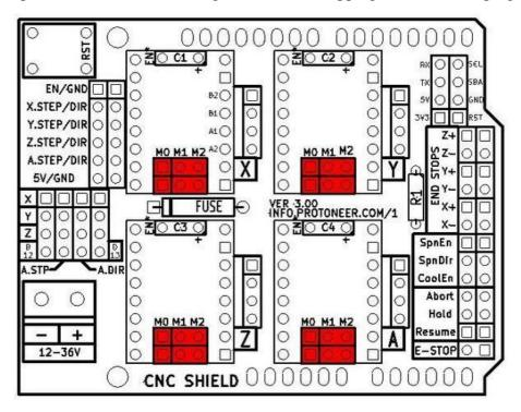
Micro-stepping jumper location, before inserting A4988.
