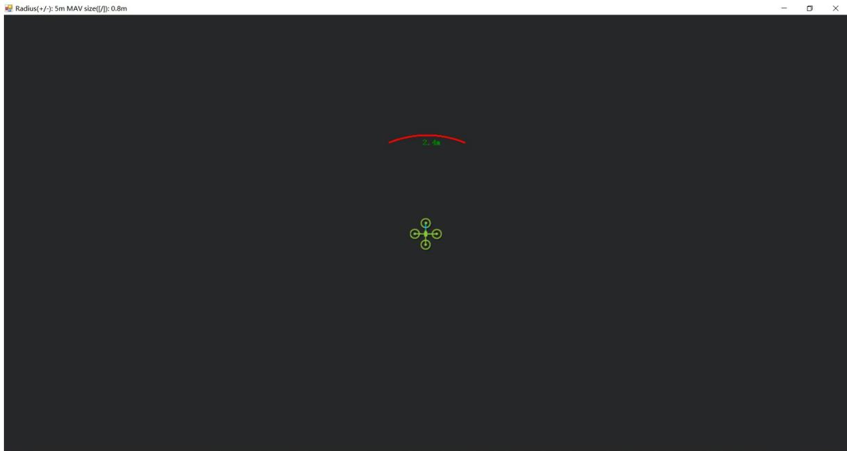
The number in green color means the distance from LiDAR in obstacle avoidance mode (the number only refresh when this window open,close,zoom in or zoom out,it doesn't mean the real time distance from LiDAR and will not be influenced in Mission Planner version under v1.3.48,the problem could be solved by updating Mission Planner)
