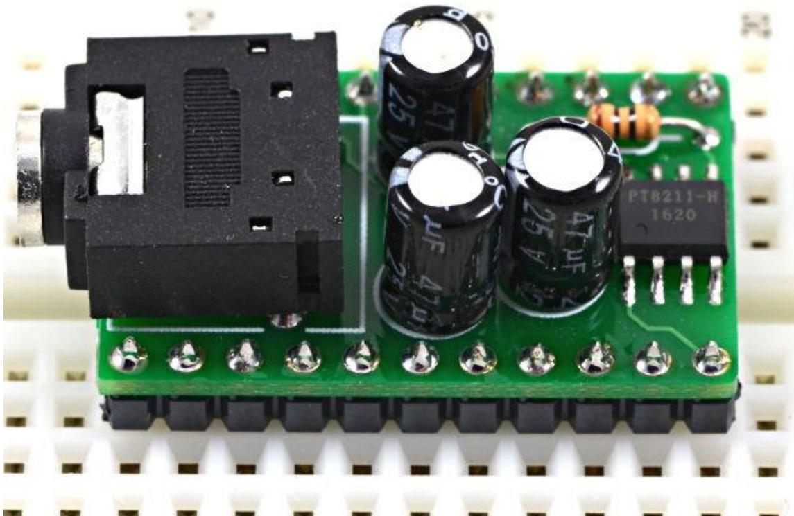
Then join your assembled PT8211 shield to your Teensy 3.2, 3.5 or 3.6. The audio connector is placed above Teensy's USB connector. The PT8211 covers 22 of the 28 pins on Teensy 3.2, or 22 of the 48 pins on Teensy 3.5 & 3.6.
