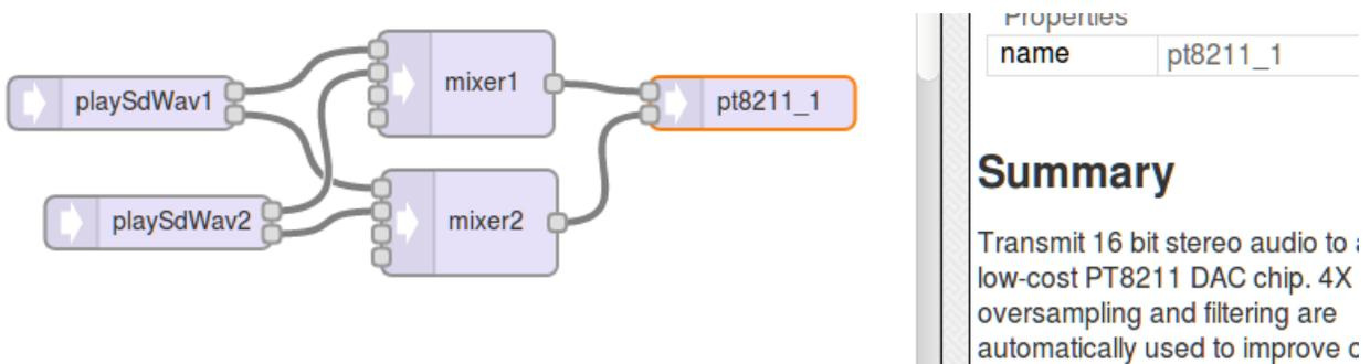
If you have code using the `sgtl5000_1` object, just delete those lines. The PT8211 has no special adjustments like volume. It simply converts digital data to analog signals.
