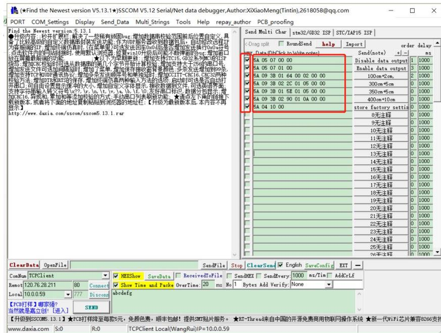
Fill in commands in this blank position (the commands refer to Chapter 4.3) and check HEX.
