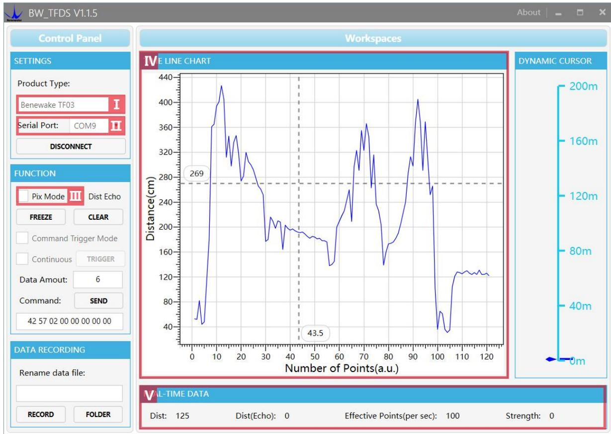
As shown in Figure 6, open the TF display program, select I 『Benewake TF03』 and select the serial port for automatic identification (here is II 『COM9』 ).
