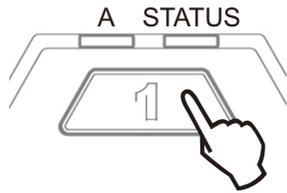
4. Press and hold the button for 3 seconds to start charging process. The status LED will be blinking with long beep.
