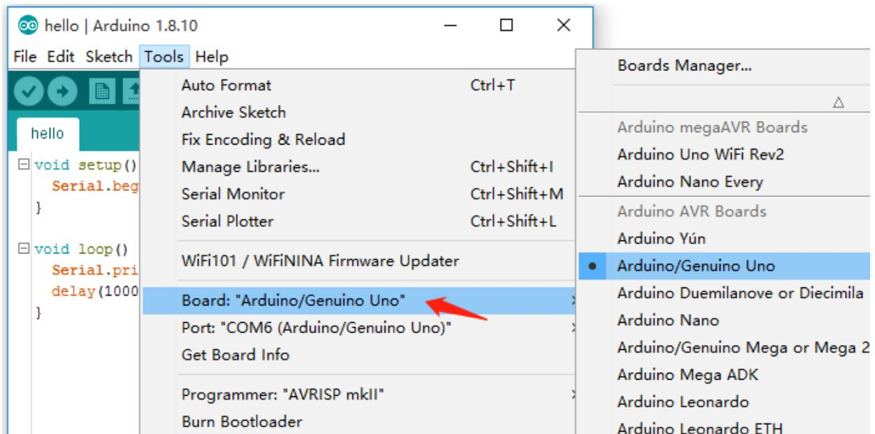
3. Click **Tools** -> **Port** to select the correct Port (the Serial Port showed in Device Manager in the previous step). In this case, **COM6** is selected. **For Mac OS users**, it should be **/dev/cu.SLAB\_USBtoUART**.
