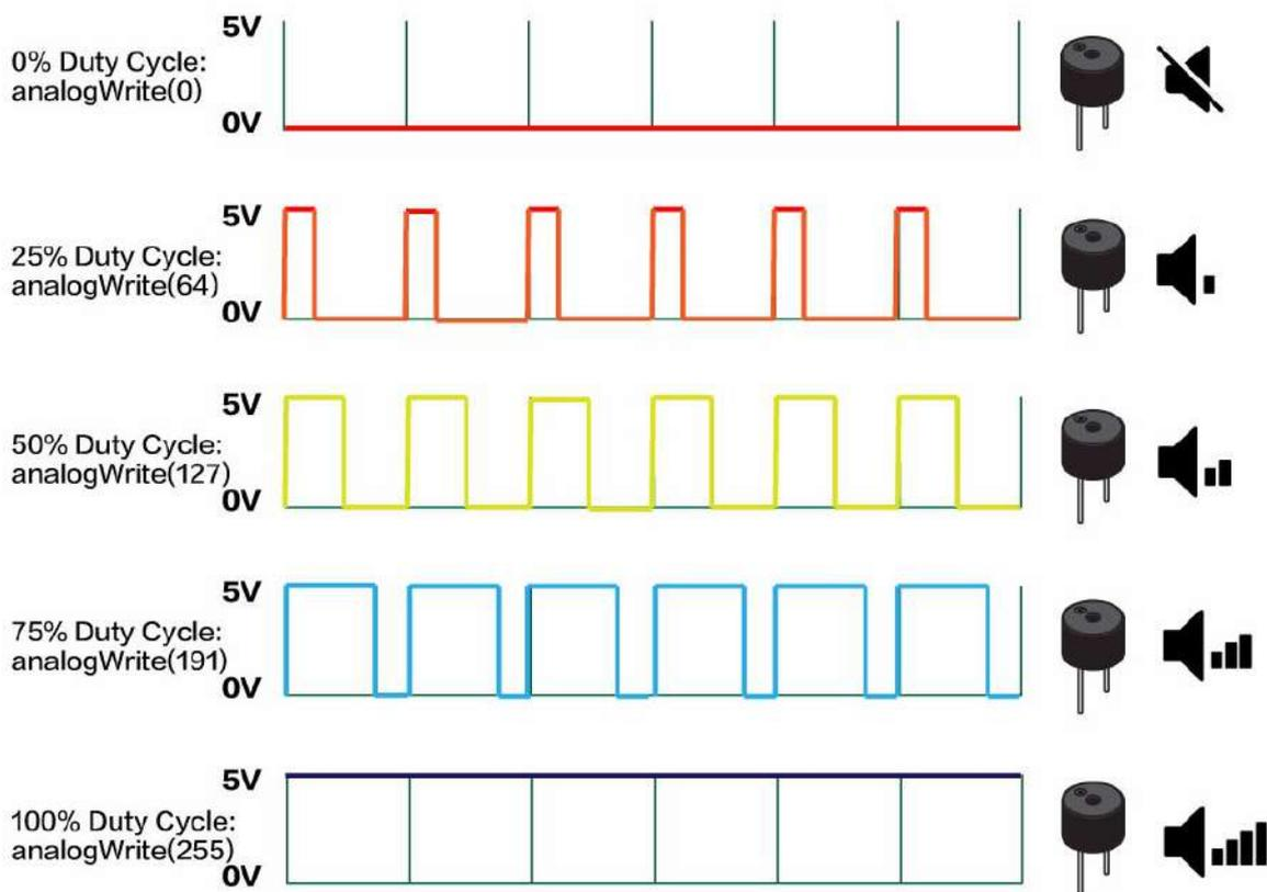
There are six digital pins on your Seeeduino that are marked with the symbol “~”, which means they can send out a PWM signal : 3,5,6,9,10,11. They are called PWM pins.
