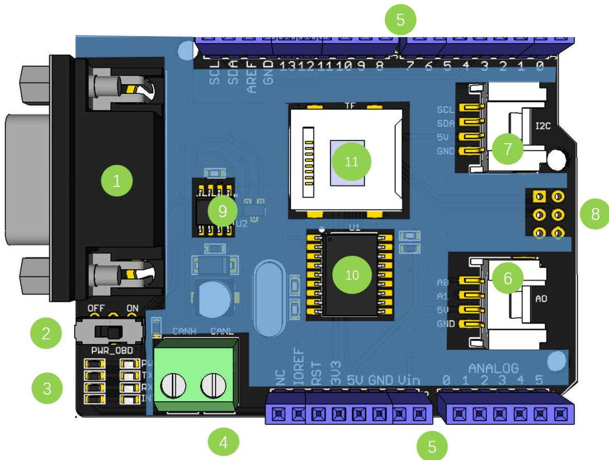
1. **DB9 Interface** - to connect to OBDII Interface via a DBG-OBD Cable.
