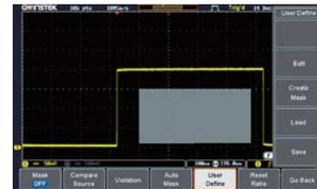
The MDO-2000A series provides the Mask function, which allows users to apply Auto Mask and user-defined Mask to determine whether the quality of the product meets the regulation. Via user-defined mask, users can set up to 8 areas and each area is up to 10 points to meet test requirements. Users can also refer to the examples from user manual to edit Mask by the PC to satisfy all test needs. By setting Save On, users can log and monitor signals, which violate test conditions.
