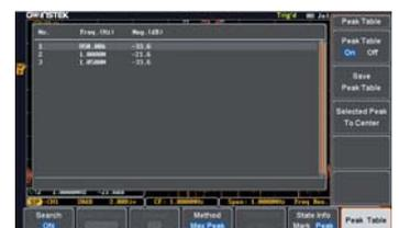
Users can use the Search function to search and mark several amplitudes and frequencies. Search methods include Max. peak and threshold. Measurement results can be displayed and saved.
