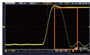
The MDO-2000A series oscilloscope allows users to easily and completely observe inrush signals and rare transient waveforms to increase waveform debugging efficiency by using features, including advanced VPO (Visual Persistence Oscilloscope) signal processing technology, waveform update rate as high as 120,000 wfm/s, and multi-layered afterglow display to enhance waveform display efficiency. Oscilloscope with VPO technology displays signals with
