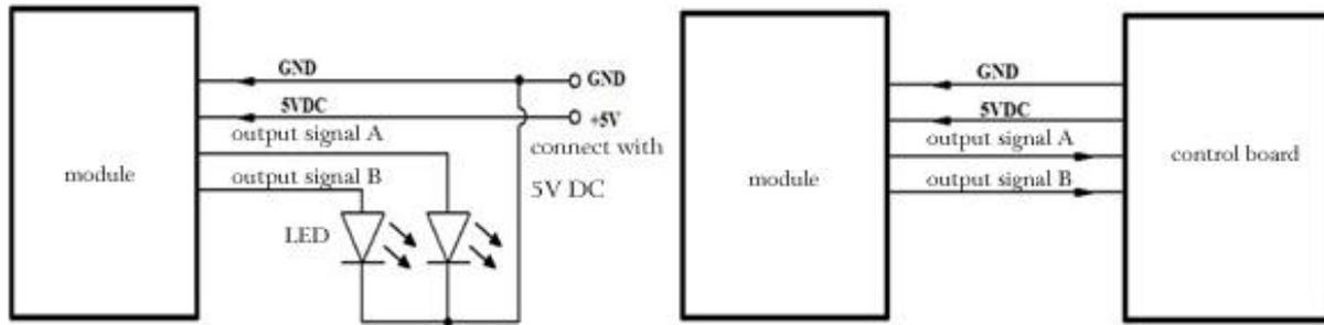
Picture 3: Module application diagram
