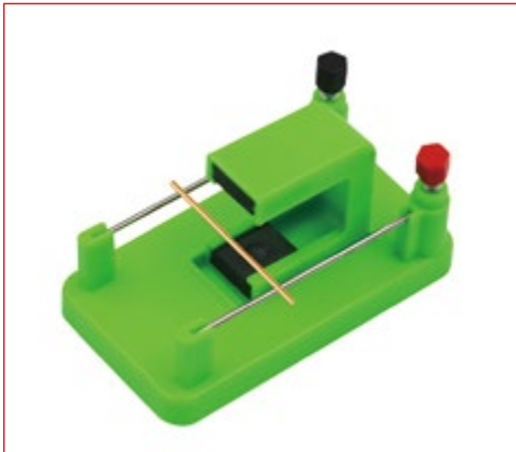
Figure 26-1 Force of magnetic field on electrical conductor
