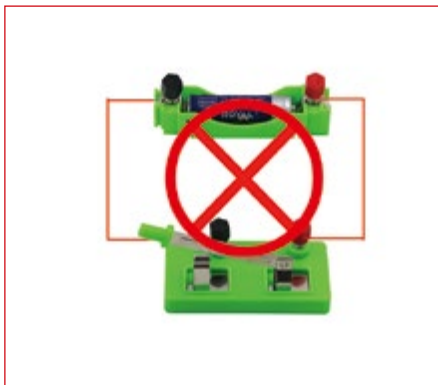
3-3 Short circuit experiment
