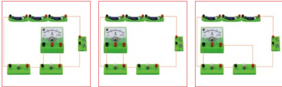
Figure 11-1 Measure voltage at both ends of L1
