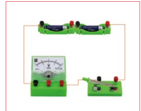
Figure 10-2 measuring battery voltage
