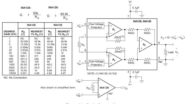
Figure 24. Basic Connections
