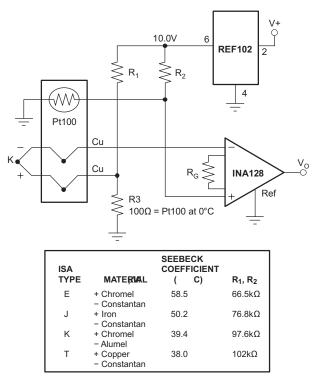
Figure 33. Thermocouple Amplifier With RTD Cold-Junction Compensation
