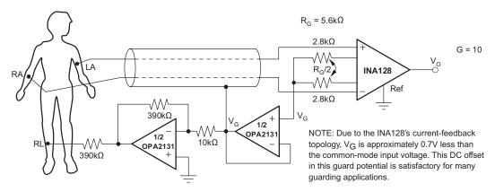
Figure 35. ECG Amplifier With Right-Leg Drive
