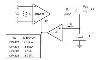
Figure 34. Differential Voltage to Current Converter
