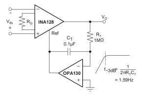
Figure 32. AC-Coupled Instrumentation Amplifier
