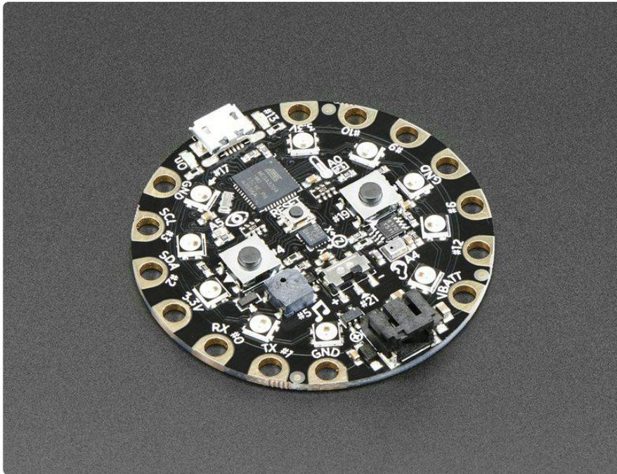
Circuit Playground has built-in USB support. Built in USB means you plug it in to program it, it just shows up - all you need is a Micro-B USB cable, no additional purchases are needed! [With the new 1.6.4+ Arduino IDE, it takes only a few seconds to add support \(https://adafru.it/nb4\)](https://adafru.it/nb4). The Circuit Playground has USB HID support, so it can act like a mouse or keyboard to attach directly to computers.
