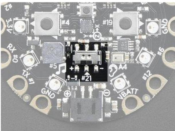
There is a single slide switch near the center of the Circuit Playground. It is connected to digital #21 and will read LOW when slid to the left, and HIGH when in the right hand position
