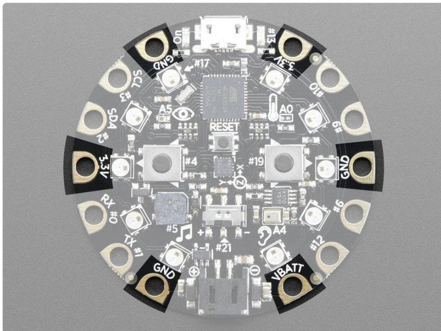
There are 6 power pads available, equally spaced around the perimeter.
