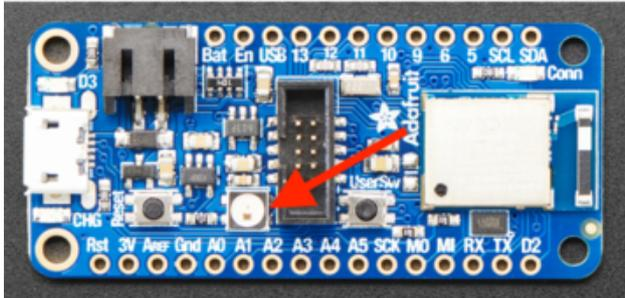
Double-click the Reset button next to the USB connector on your board, and you will see the NeoPixel RGB LED turn green (identified by the arrow in the image). If it turns red, check the USB cable, try another USB port, etc. Note: The little red LED next to the USB connector will pulse red. That's ok!
