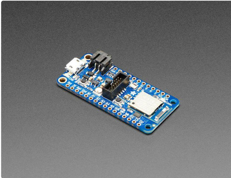
For this chip, we've added Arduino IDE support - you can program the nRF52840 chip directly to take full advantage of the Cortex-M4 processor, and then calling into the Nordic SoftDevice radio stack when you need to communicate over BLE. Since the underlying API and peripherals are the same for the '832 and '840, you can supercharge your older nRF52832 projects with the same exact code, with a single recompile!
