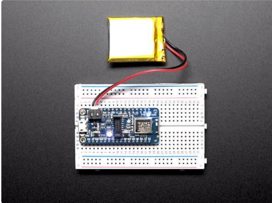
The Adafruit Feather nRF52840 Express is the new Feather family member with Bluetooth Low Energy and native USB support featuring the nRF52840! It's our take on an 'all-in-one' Arduino-compatible + Bluetooth Low Energy with built in USB plus battery charging. With native USB it's even ready to join the CircuitPython party. [We have other boards in the Feather family, check'em out here. \(https://adafru.it/l7B\)](https://adafru.it/l7B)
