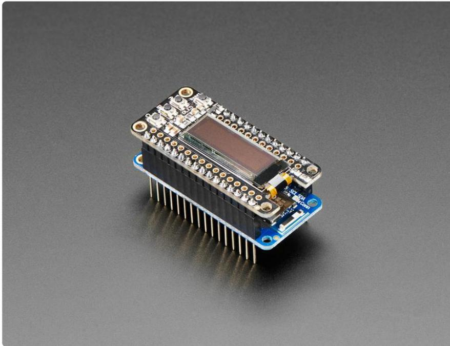
It's got tons of awesome peripherals: plenty of GPIO, analog inputs, PWM, timers, etc. Best of all, it's got that native USB! Finally, no need for a separate USB serial chip like CP2104 or FT232. Serial is handled as a USB CDC descriptor, and the chip can act like a keyboard, mouse, MIDI device or even disk drive. (Note that we don't have support for anything but CDC for Arduino at this time)
