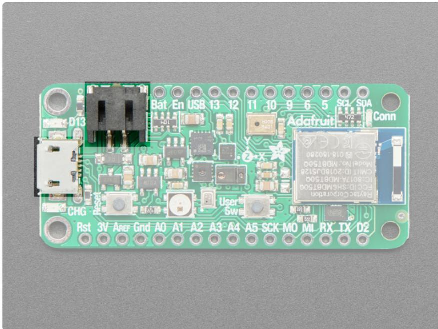
The above shows the Micro USB jack (left), LiPoly JST jack (top left), as well as the changeover diode (just to the right of the JST jack) and the LiPoly charging circuitry (to the right of the JST jack).
