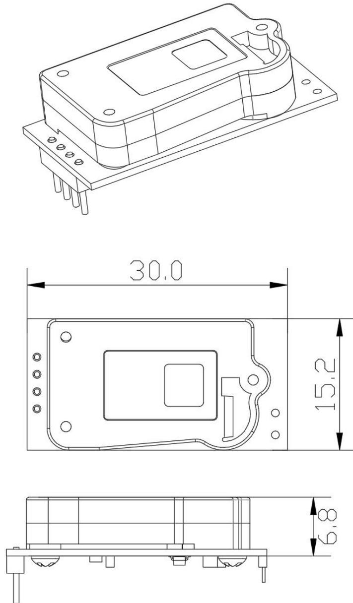
. Figure 4 ACD10 dimensions (unit: mm)
