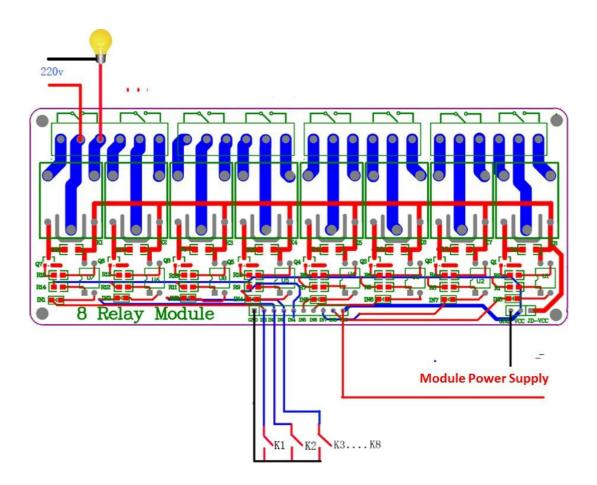
It is sometimes possible to use this relay boards with 3.3V signals, if the JD-VCC (Relay Power) is provided from a +5V supply and the VCC to JD-VCC jumper is removed. That 5V relay supply could be totally isolated from the 3.3V device, or have a common ground if opto-isolation is not needed. If used with isolated 3.3V signals, VCC (To the input of the opto-isolator, next to the IN pins) should be connected to the 3.3V device's +3.3V supply.
