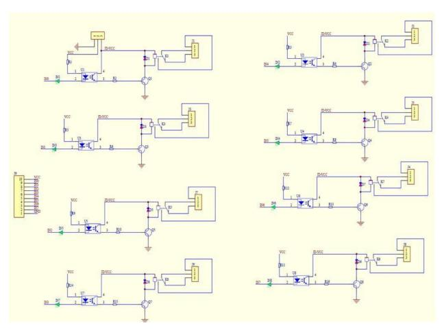
**8 Channel Relay Module Schematic**
