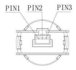
PIN1 +5V PIN2 PT PIN3 IR\_ADJ
