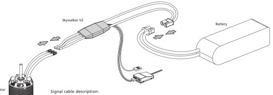
Throttle Signal Cable (White/Red/Black Tri-color Cable): plug it into the TH channel on the receiver or flight controller. The White wire is for transmitting throttle signals, the Red & Black wires are BEC output wires.
