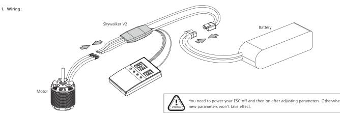
1). Plug the programming cable (on your ESC) into the programming port on the LED program box.
