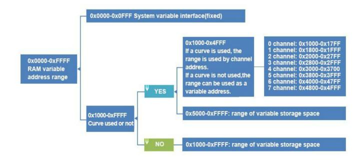
The variable address is the first address of the subspace in which one or more variables are stored in the RAM space, and the code of the display variable or the value of the state variable is stored in the space pointed to by this address.
