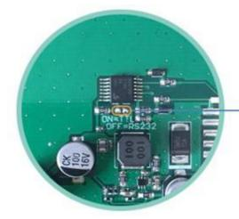
ON: short circuit, TTL level OFF: disconnect, 232 level 232 level is not connected by default
