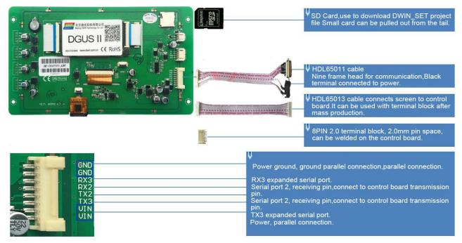
8pin2.0 interface definition and wiring
