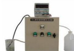
Hypochlorite water generator
