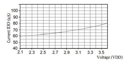
Figure 6 Typical supply current vs. supply voltage curve (sleep mode) at a temperature of 25  $^{\circ}$ C. Note: The deviation between these data and the displayed value may reach ±50% of the displayed value. At 60  $^{\circ}$ C, the coefficient is approximately 15 (compared to Table 3).
