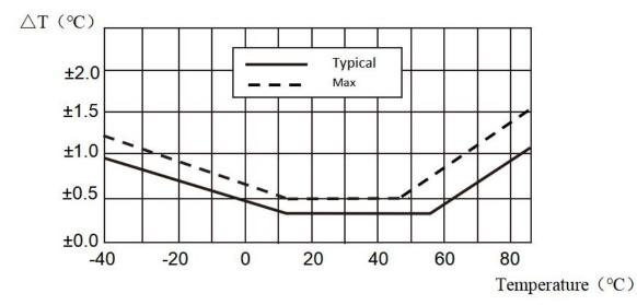
Figure 2 Temperature typical error and maximum error
