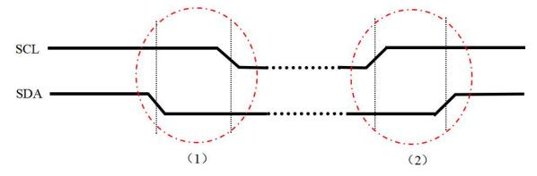
Figure 11 Start transmission state (S) and stop transmission state (P)
