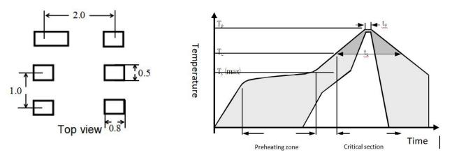
Figure 8: Recommend WHT 20 PCB design size (unit: mm), the outer dotted line part is the external size of the SMD package.
