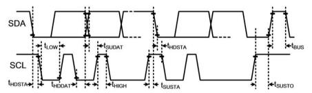
Figure 10 The timing diagram and abbreviations of the digital input/output terminals are explained in Table 7. The thicker SDA line is controlled by the sensor, and the ordinary SDA line is controlled by the microcontroller. Please note that the SDA valid read time is triggered by the falling edge of the previous conversion.
