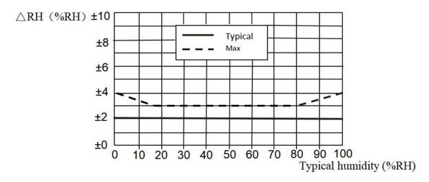
Figure 1 Maximum error of relative humidity at 25°C
