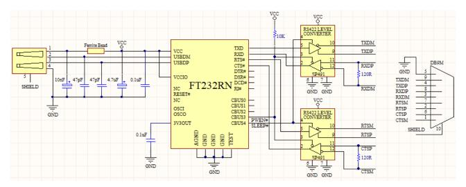
Figure 7.3 USB to RS422 Converter Configuration
