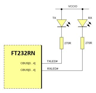
Figure 7.5 Dual LED Configuration
