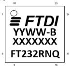
The date code format is **YYWW-B** where WW = 2-digit week number, YY = 2-digit year number, B = singleletter corresponding to the revision of the device (e.g., A or B or C).
