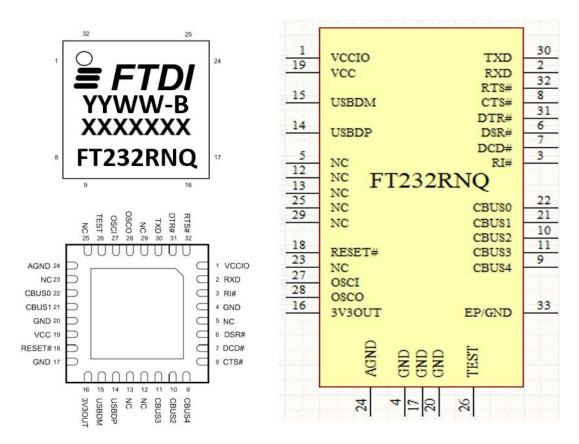
Figure 3.2 QFN-32 Package Pin Out and schematic symbol
