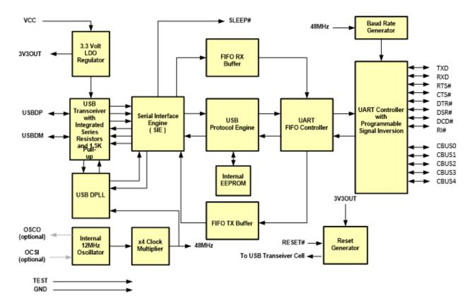
Figure 2.1 FT232RN Block Diagram
