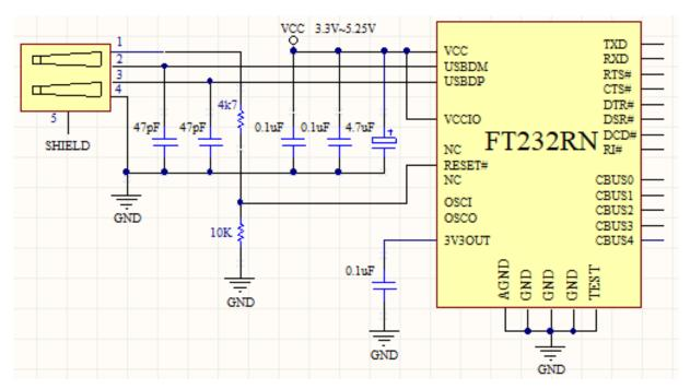
Figure 6.2 Self-Powered Configuration
