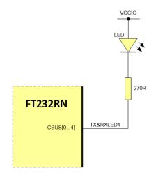
Figure 7.6 Single LED Configuration
