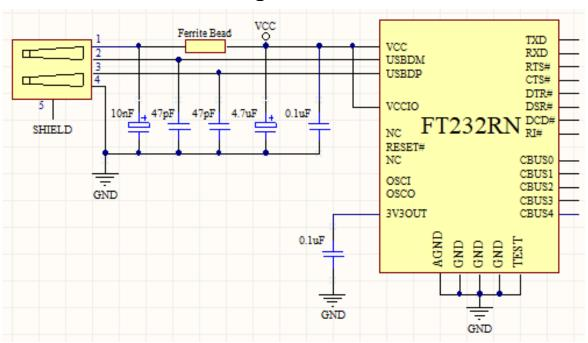
Figure 6.1 Bus Powered Configuration
