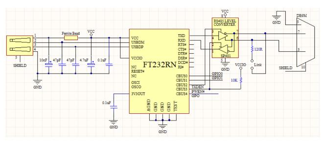
Figure 7.2 Application Example Showing USB to RS485 Converter
