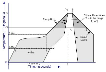
Figure 9.3 FT232RN Solder Reflow Profile
