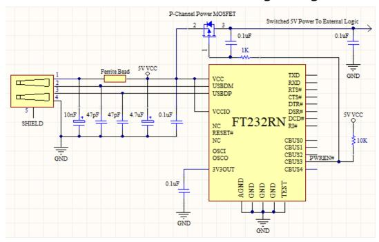
Figure 6.3 Bus Powered with Power Switching Configuration
