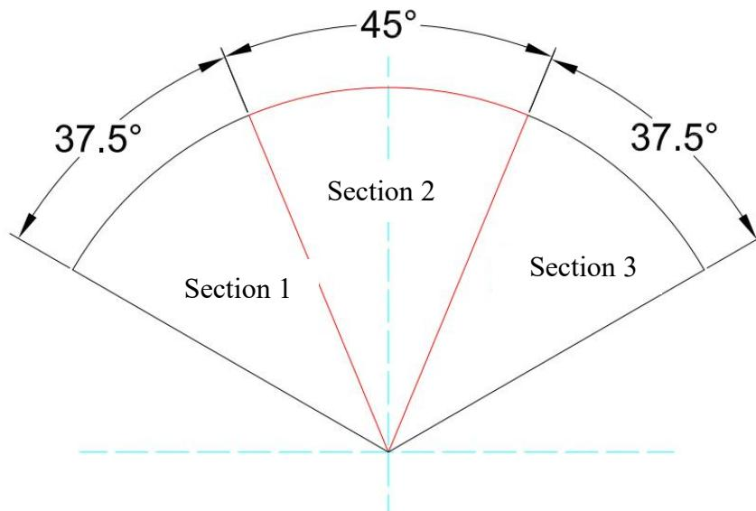
3. If the version is three-sector, it will only output the nearest target of the three-sector. The output order is sector 1, sector 2, and sector 3. If the sector has no target, the distance velocity value will be assigned to 0.
