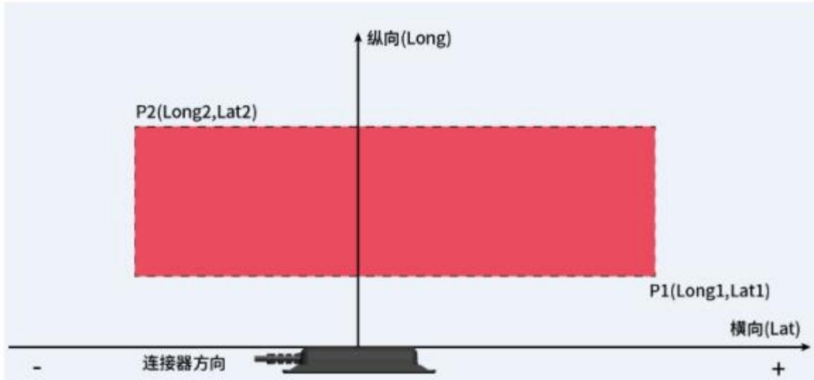
Now support set only one input rectangle, two coordinates points P1, P2 determine a rectangle region, and to set detected objects output numbers on this region, allow output number is “N”, if “N” is greater than the number of actual detected objects in the rectangle region, then the actual number is output; If “N” is less than the number of actual detected objects in the rectangle region, then the “N” is output.(Output in order of distance near to far).
