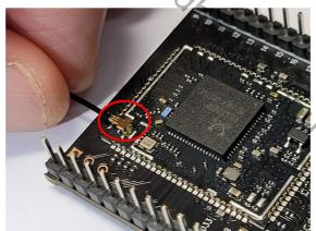
Step 3: Push cable connector at center location vertically. The connectors mating action is completed when click sound could be heard.
