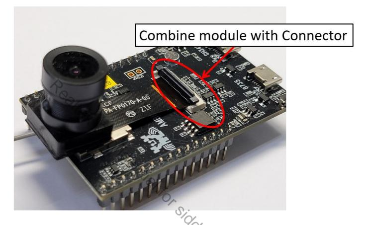
Step 4 : Close the connector carefully and make sure that the lens of sensor module is clear.
