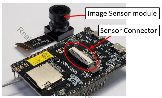
Step 2: Open sensor connector carefully.
