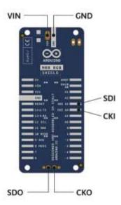
As you may know, each LED RGB SMD chip can draw up to 40 mA. If we multiply the maximum current by the number of LEDs we get to close to 4A. This is the peak current with all the LEDS set to white and full brightness. Nothing that the MKR regulator or a standard PC USB port can support, therefore the shield has a separate power supply connector, capable of handling up to 4A. Please connect a proper 5V power supply to the shield if you plan to create dense graphics at high brightness.
