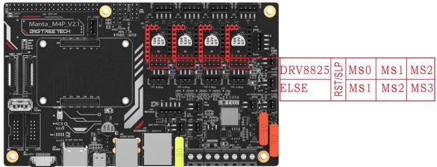
Note: If using A4988or DRV8825, RST and SLP must be shorted with jumper caps for normal operation.
