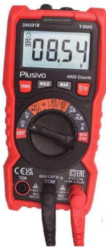
The measured voltage in this figure is 8.54 V DC.
