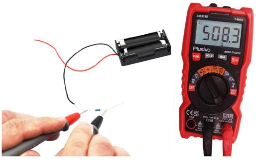
The measured resistance in this figure is 508.3  $\Omega$
