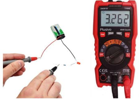
The measured current in this figure is 3.262 mA.
