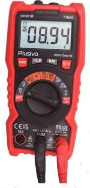
The measured voltage in this figure is 8.94 V DC.
