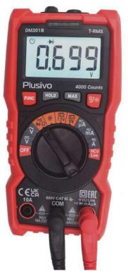
The measured forward voltage in this figure is 0.672 V.
