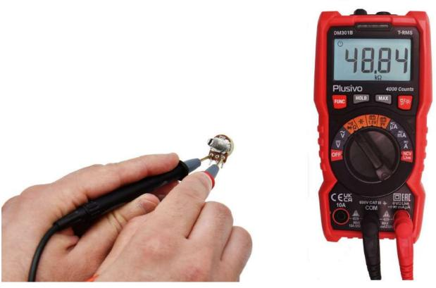
The measured resistance in this figure is 48.84  $\mbox{k}\Omega.$
