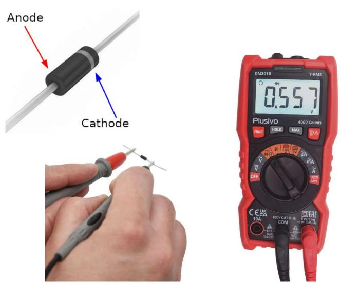
The measured forward voltage in this figure is 0.557 V
