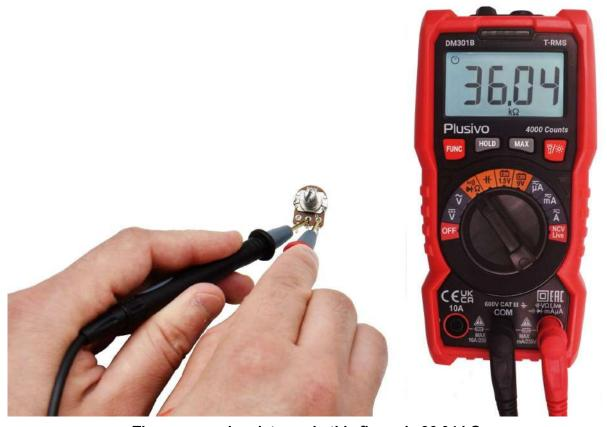
The measured resistance in this figure is 36.04  $k\Omega.\,$
