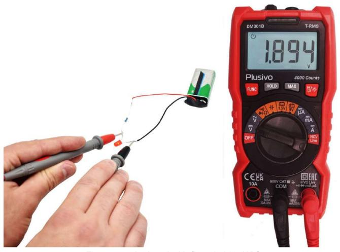
The measured voltage in this figure is 1.894 V DC
