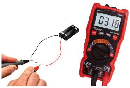
The measured voltage in this figure is 3.18 V DC.
