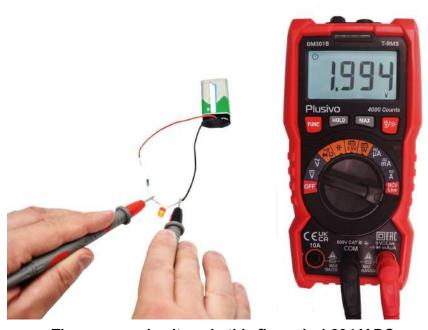
The measured voltage in this figure is 1.994 V DC
