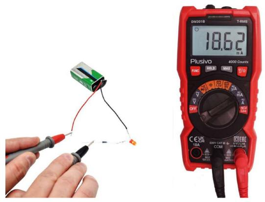
The measured current in this figure is 18.62 mA.
