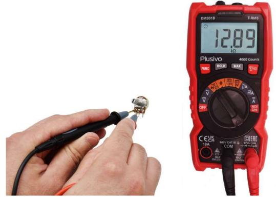
The measured resistance in this figure is 12.89  $k\Omega.\,$
