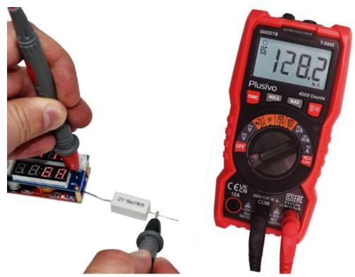
The measured current in this figure is 128.2 mA
