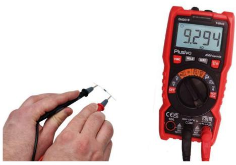
The resistance measured in this figure is 9.294  $k\Omega$
