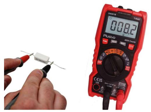
The measured resistance in this figure is 8.2  $\Omega$ .
