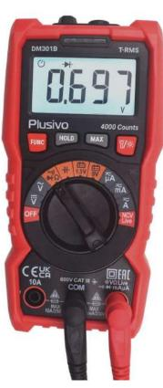
The measured forward voltage is 0.697 V.
