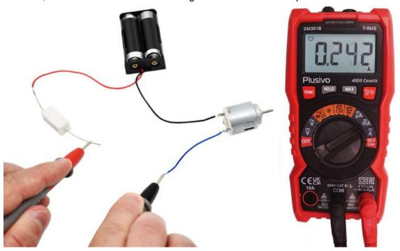
The measured current in this figure is 242 mA.
