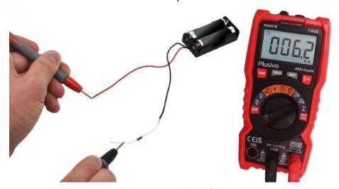
The measured current in this figure is 6.2 mA
