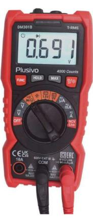
The measured forward voltage is 0.691 V.
