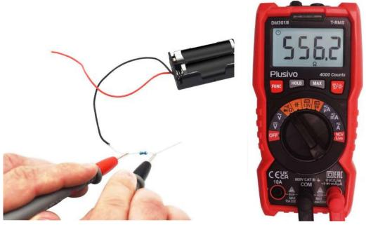
The measured resistance in this figure is 556.2  $\Omega$ .
