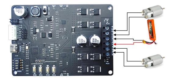
SmartElex 10D can be used with power supplies or batteries. Input power is connected to the center power terminals labeled VIN and GND. The input voltage range is 7V to 22V. The input current is dependent on the motors being used and the load placed upon them.
