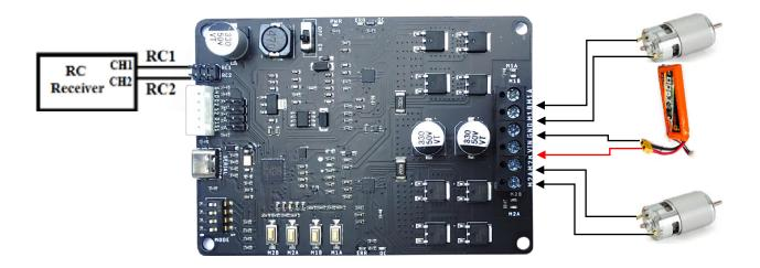
Sample Connection Diagram of RC receiver and motor with SmartElex 10D.
