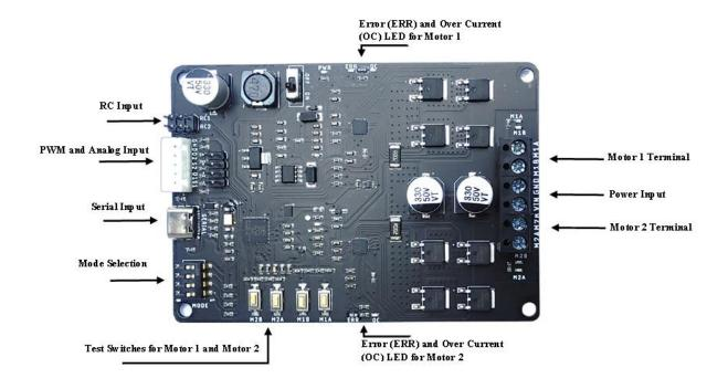
**Power Input**: Connect to a 7V-22V Battery or Power Supply.
