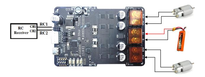
Sample Connection Diagram of RC receiver and motor with SmartElex 30D.
