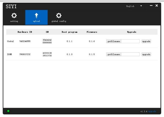
4. If the firmware is not latest, then click the "Select File" button in the "Gimbal" to import the latest firmware. And click "Upgrade" and wait till it is "100%" finished.
