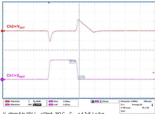
Figure 26: Load transient ( V_{OUT} = 1.2\text{ V} )
