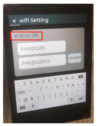
After successfully connecting to WiFi, the time will be updated to Beijing time synchronously. Note: the time required to restart the module will be re-timed, and WiFi needs to be re-entered.
