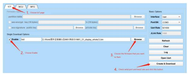
COM Port: Select the COM port number connected to the chip (if there is no COM port displayed, click the "Refresh" button to refresh the COM port option), select 921600 for Uart Rate, click the "Create & Download" button to start downloading the firmware, when "ALL Success" is displayed, It means that the firmware download is complete.
