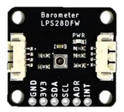
The Absolute Digital Barometer - LPS28DFW offer a unique barometer breakout featuring the LPS28DFW from STMicroelectronics<sup>©</sup>. The LPS28DFW is an absolute barometer with a water-resistant package making it perfect for pressure measurement applications where the sensor is exposed to or even submerged in water<sup>1</sup>.
