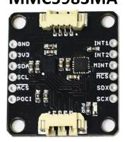
The MMC5983MA combines the high-performance ISM330DHCX 3D digital accelerometer and gyroscope from STMicroelectronics with the highly sensitive triple-axis magnetometer by MEMSIC to give you an ultra powerful, easy to use breakout board.
