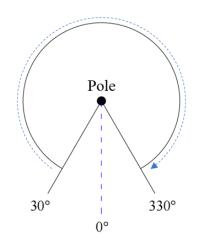
FIG 4 YDLIDAR TEA POLAR COORDINATE SYSTEM DEFINITION
