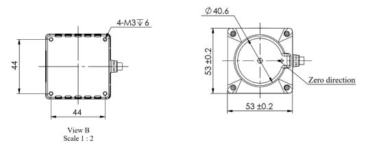
FIG 1 YDLIDAR TEA INSTALLATION DIMENSION (UNIT:MM)
