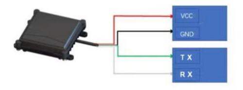
Picture 4 Serial port line connection
