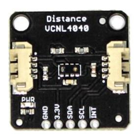
We often see this type of sensor on automatic towel dispensers, automatic faucets, etc. However, the VCNL4040 has **no dead zone** and can read all the way up to the face of the sensor. The Proximity VCNL4040 sensor is a great digital alternative to the popular analog PIR sensors. The Proximity Sensor also has an ambient light sensor built it which is excellent if you need a digital light sensor.
