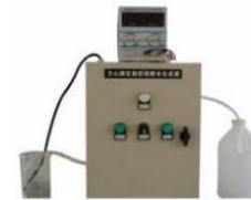
Hypochlorous Acid Generator
