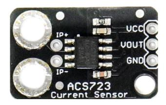
The ACS723 sensor uses a Hall effect sensor to output a voltage relative to the current flowing through the IP+ and IP- pins. The advantage of using a Hall effect sensor is that the circuit being sensed and the circuit reading the sensor are *electrically isolated*. This means that, although your Arduino is running on 5V, the sensed circuit can be operating at higher DC or AC voltages!
