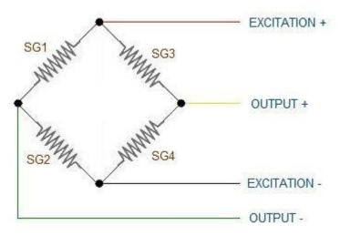
*Four strain gauges (SG1 through 4) hooked up in a wheatstone bridge formation* The four wires coming out from the wheatstone bridge on the load cell are "usually":
