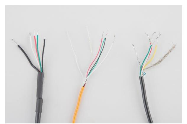
Here we have a large black wire, some loose wires, and foil and loose wires respectively as EMI buffers In general, each load cell has four strain gauges that are hooked up in a **wheatstone bridge** formation as shown below.
