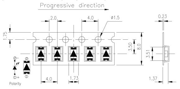
Note: The tolerances unless mentioned is  $\pm 0.1$ mm ,Unit = mm **Moisture Resistant Packaging**
