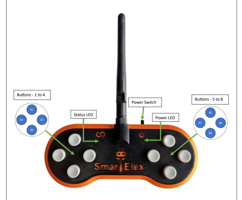
**Status LED** is always on indicating the transmitter and receiver are communicating with each other.
