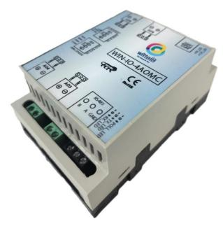
The IO modules are mounted on DIN rail mountable casing and with exposed connectors and LED indicators. The DIP switch for Slave ID and Baud rate are placed inside the enclosure. (Soft setting option is also available)
