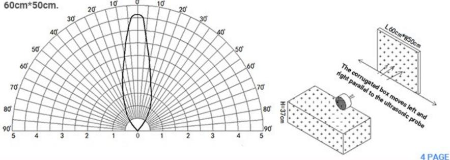
(3) The tested object is a corrugated box tangent to the arc, length \* width is 60cm\*50cm.
