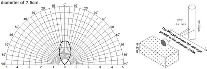
(2) The tested object is a corrugated box perpendicular to the 0° central axis, with a length \* width of
